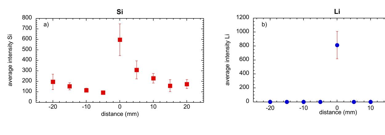
Average intensities of (a) silicon, (b) lithium in Dogger limestone as a function of the distance to the stylolite.
