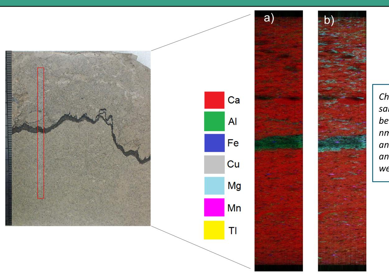
Chemical maps by LIBS of a sample of Dogger limestone between wavelengths of 250 nm and 300 nm: (a) Ca, Al, and Fe, (b) Ca, Al, Cu, Mg, Mn and Ti. Silicon and lithium were not visible in this range.
