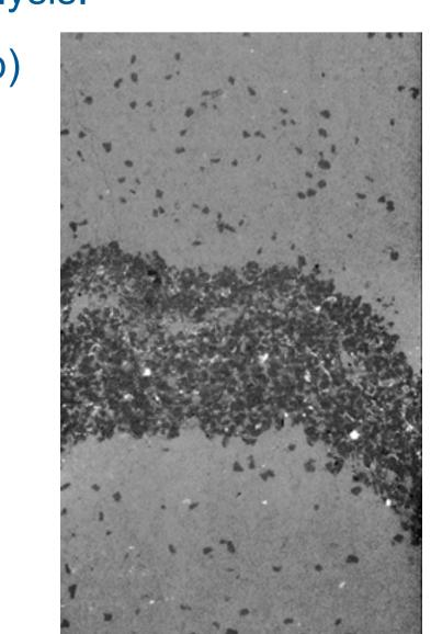
(a) Studied stylolite in a limestone of Dogger age. (b) Xray Computed microtomography data (CT) with 4  $\mu$ m resolution on the same sample. The thickness of this part of the stylolite was about 2 mm. Quartz grains appear darker in the CT data.
