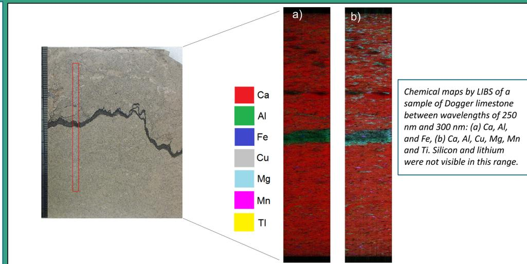
Chemical maps by LIBS of a sample of Dogger limestone between wavelengths of 250 nm and 300 nm: (a) Ca, Al, and Fe, (b) Ca, Al, Cu, Mg, Mn and Ti. Silicon and lithium were not visible in this range.
