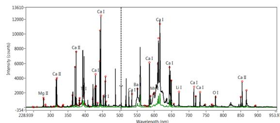
Example of spectrum on the Dogger limestone for a single shot (black) and an average of 50 shots (green). Peaks of calcium (Ca) and magnesium (Mg) are visible at this scale. Zooming on such data gave the precise composition of the sample.
