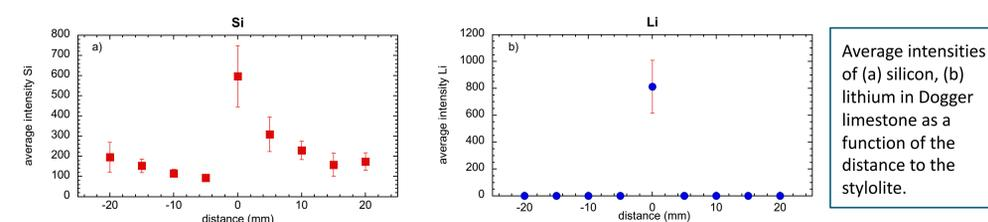
Average intensities of (a) silicon, (b) lithium in Dogger limestone as a function of the distance to the stylolite.
