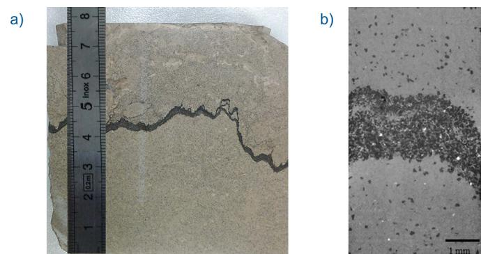
(a) Studied stylolite in a limestone of Dogger age. (b) X-ray Computed tomography data (CT) with 4 μm resolution on the same sample. The thickness of this part of the stylolite was about 2 mm. Quartz grains appear darker in the CT data.
