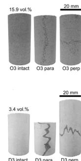
Compilation of permeability on carbonates from Lind et al. (1994), Heap et al. (2012) and Rustichelli et al. (2015). Measurements were performed on stylolite-free samples and on samples with a stylolite oriented parallel and perpendicular to flow (blue triangles). When oriented orthogonal to flow, stylolites had no effect on permeability.
