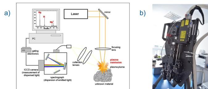
a) A typical laboratory LIBS set-up (from <https://www.uni-muenster.de/Planetology/en/ifp/research/geologischeplanologie/LIBS.html>). b) Photograph of the LIBS system of Epitopos.
